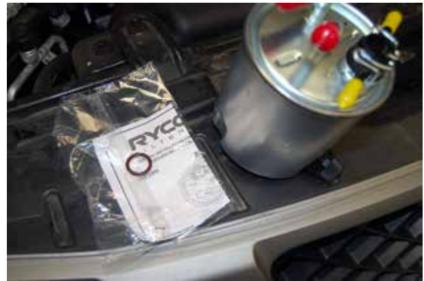
2. Replace the old o-ring with the new one supplied, to the water sensor.
