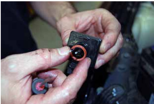
3. Make sure the gasket sits properly in the groove and that it is not damaged.
