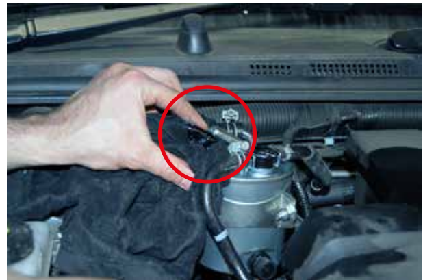
4. Prime the filter until a clean stream of fuel comes out of the filter's outlet.
